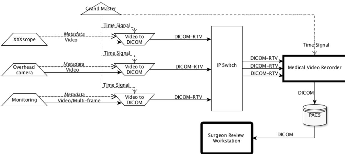
**Figure PPP.3-1: Recording multiple video sources**
