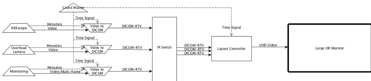
**Figure PPP.4-1: Displaying multiple source on one unique monitor**
