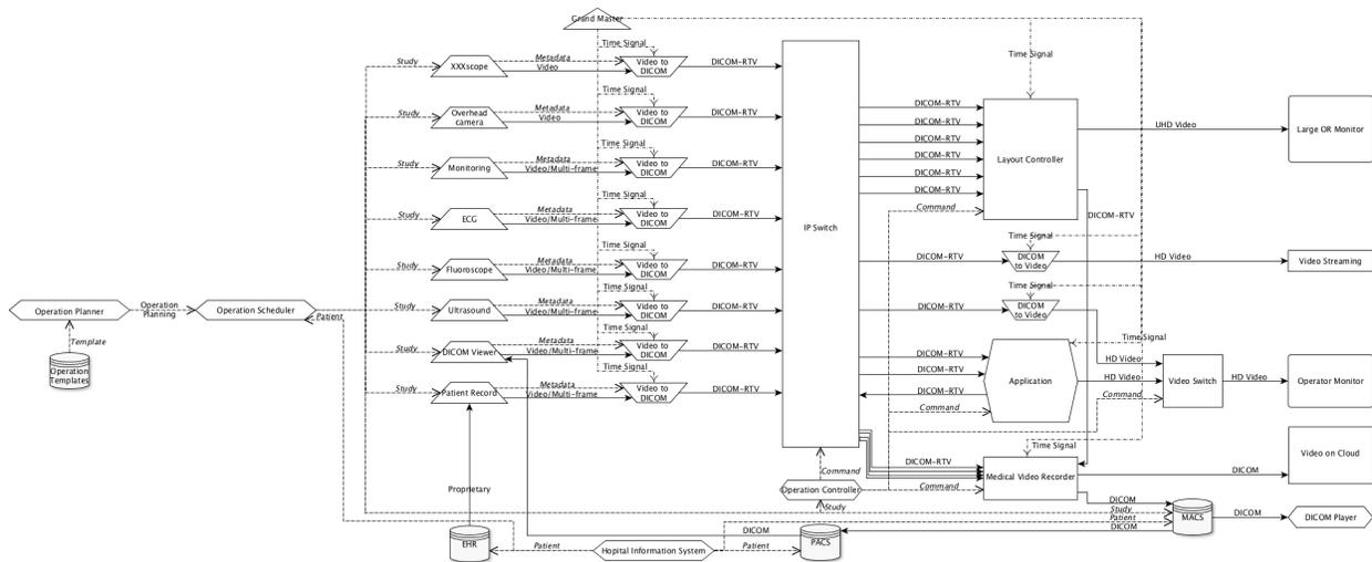
Figure PPPP.1-1: Overview diagram of operating room
