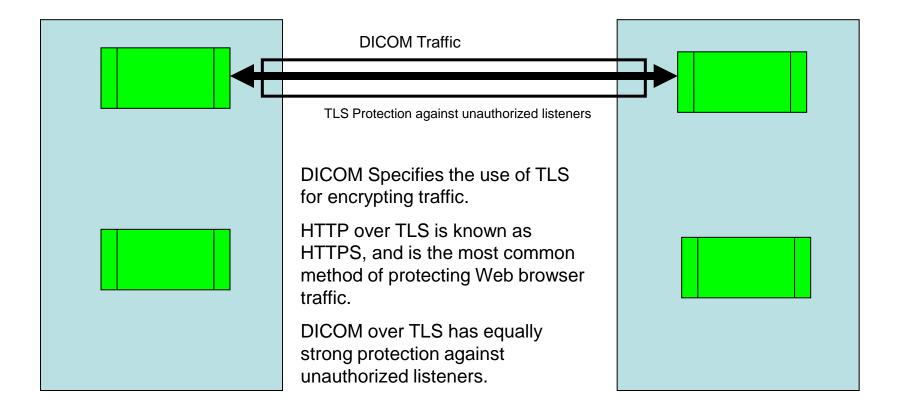
Protection against unauthorized network listeners by means of encryption
